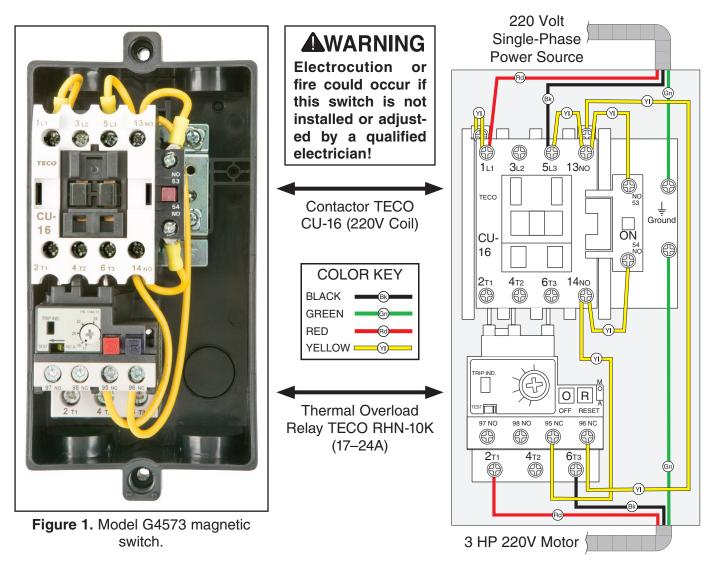
**IMPORTANT:** This magnetic switch toggles a motor ON and OFF, and helps provide thermal overload protection for the motor if the operating temperature gradually increases due to heavy work loads. The thermal overload relay inside is not designed to cut power in the event of a sudden motor overload or stall. To help protect a motor from this type of overload, the power supply circuit must be properly sized for the full-load current rating of the motor.
